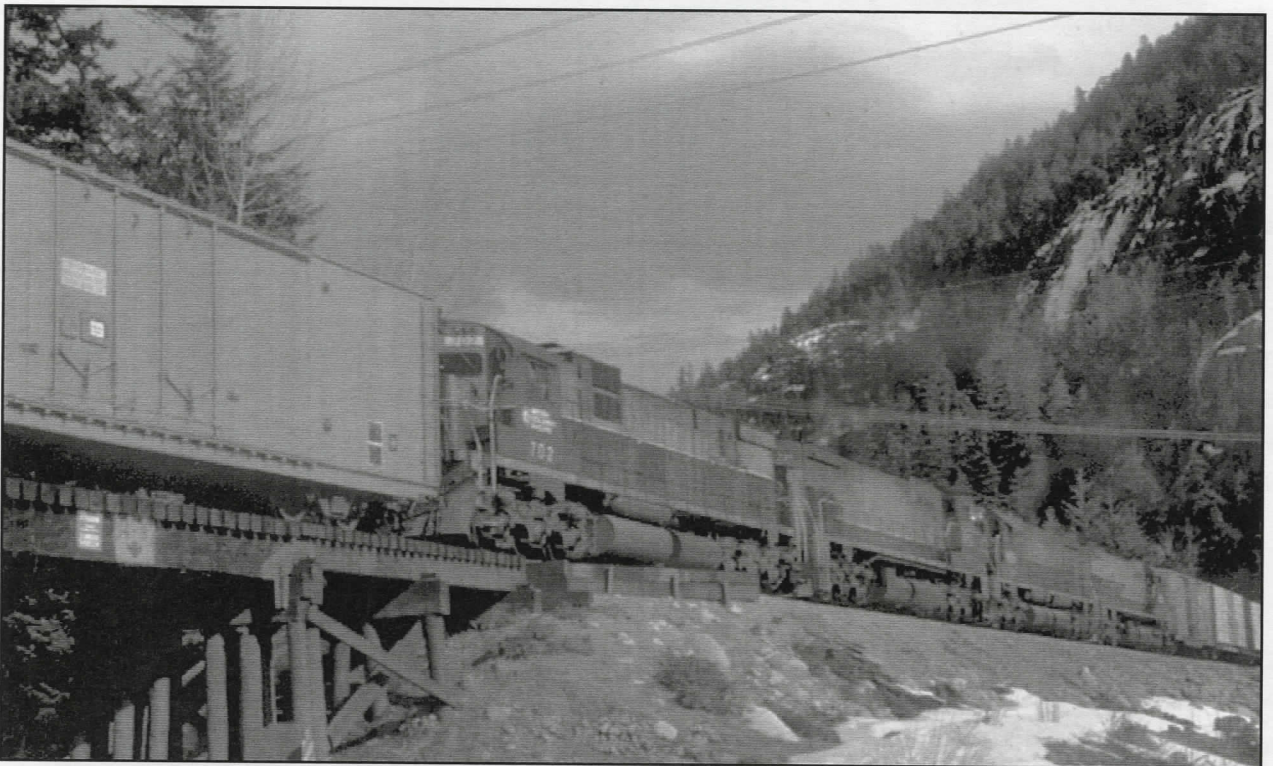
56 cars back from the head end consist were four more 630s working that week on the "Pemberton Push". C630#702, M630W 730, M630 706 and M630 709 are shoving hard on the grade. The pushers were cut into the train at Darcy and will be cut out at Mons. Interestingly, this crew would swap out some of the pusher power at Mons, as #14 traded the 726 for 702 and 730 from the pusher set.
