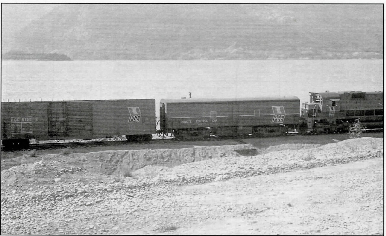
The railway began its Locotrol operations in 1970 with the use of robot cars coupled to the mid-train locomotives. RCC 2 is seen mid-train at Porteau in June 1973.
