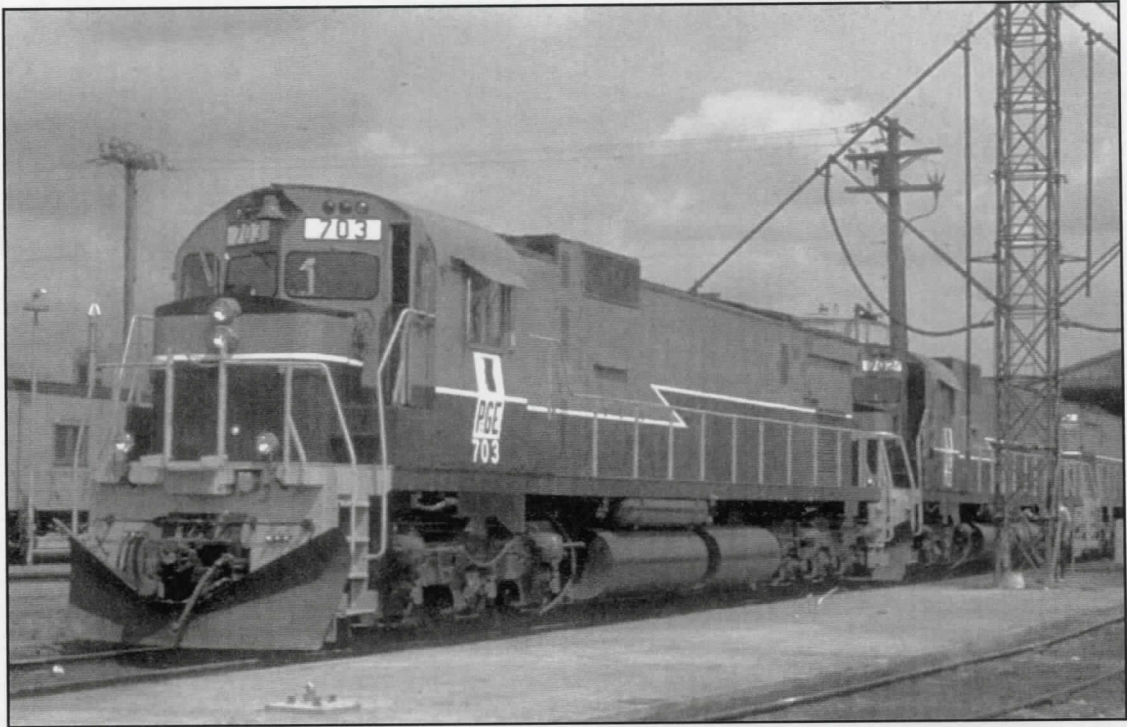
C-630M Nos. 703, 702 and 701 are seen at the North Vancouver diesel shop shortly after delivery on August 2, 1969. The horns have yet to be relocated above the bell.
