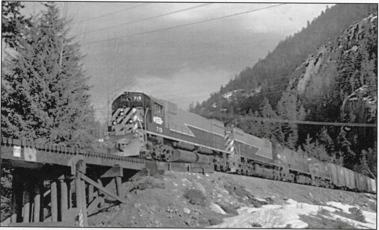
The sound of screaming Alco 251 fills the air as Train No. 14 slugs its way up the 2.2% grade through Tisdall on 11 March, 1985. Over 22,000 hp is needed on this day to push and pull the loads over the grades south of Darcy. Up front are M630 #719, M630W #726, M420B #RCL681 and C425 #807. Interestingly, #726 was the first unit to receive the final version of the two tone green paint scheme and #719 was the last of the 630s to receive it.
