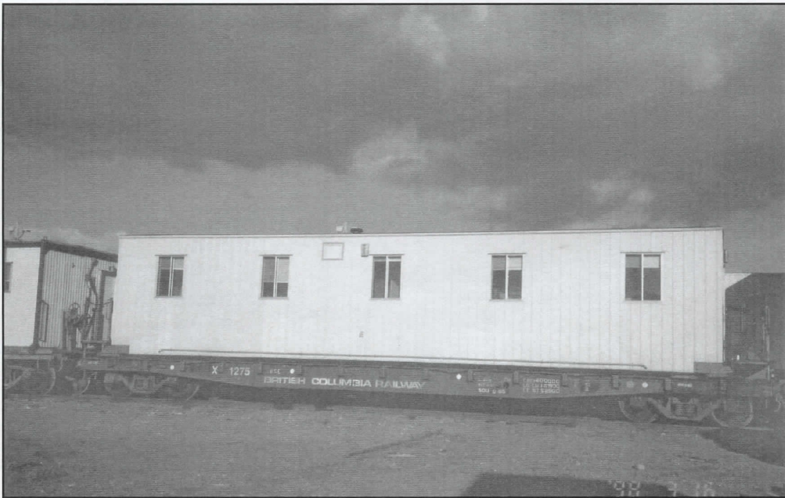
Fig. 7 BCOL X-1275 is one of more than two dozen standard flatcars which were fitted with Scotia trailers for outfit service. Note the platforms and handrails at each end of the car. An outfit train could consist of 4-8 of these cars. Photograph by Andy Barber
