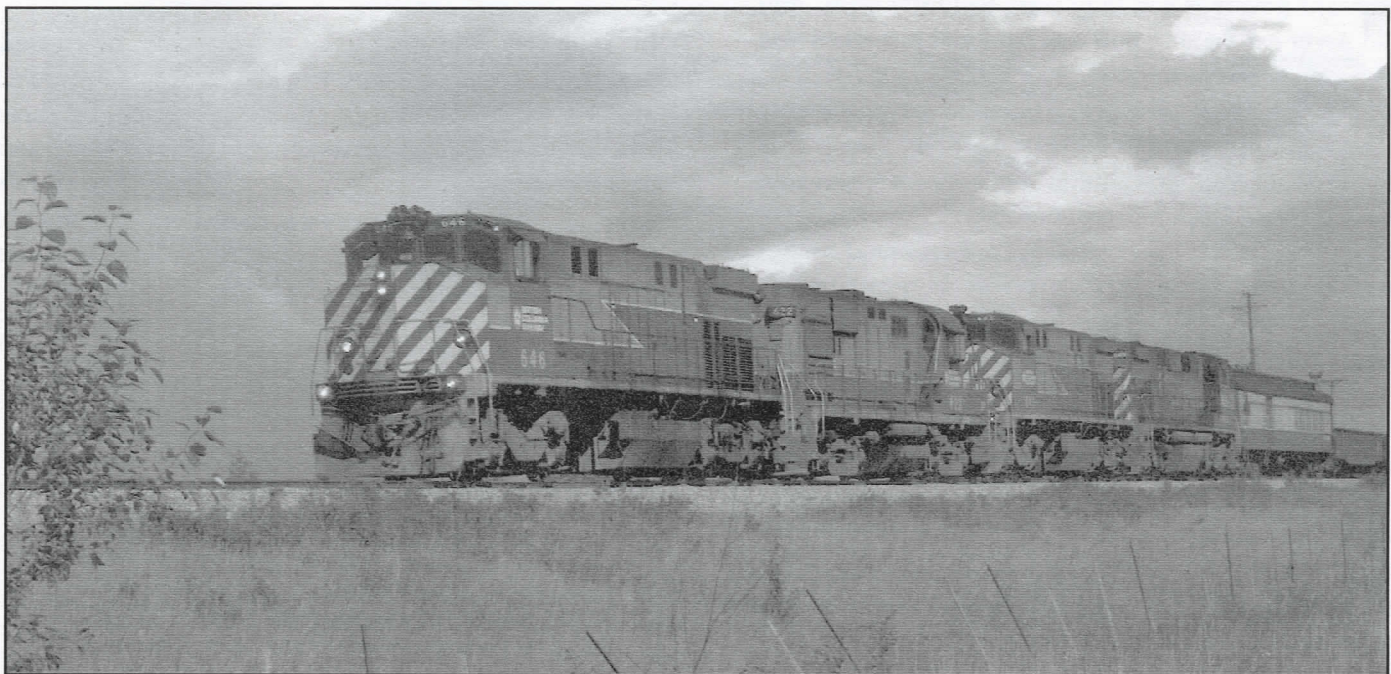
Fig. 4 Under threatening skies, Extra 646 North departs Fort St John BC on the afternoon of 20 August, 1987. Three M420s and an RS-18 are the power for the up one day, back the next train to Fort Nelson B.C. From its opening, Nelson Subdivision trains were always powered with four axle locomotives due to poor track and the need for lighter axle-loadings. In the late 1980s the railway set out to upgrade the Nelson and Fort St John Subdivision trackage to allow the larger six axle locomotives to operate there. The old combine behind the power on this train was used to ferry work crews to points up the line not accessible other than by rail. By the 1990s the trackwork would be done and locotrol-equipped SD40-2s would hold down the road jobs on the Nelson Sub and the M420s would be assigned elsewhere. 646-622-643-645 and 43 cars. Photograph by B.A. Elchlepp
