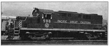
brakes, roller type wheel bearings and lightweight trucks. (The trucks were later replaced with regular ones or swapped with Rs-3 and RS-10 trucks. The main spotting feature is the lightweight ones did not have leaf springs in the middle. Refer to photos for accuracy.)
