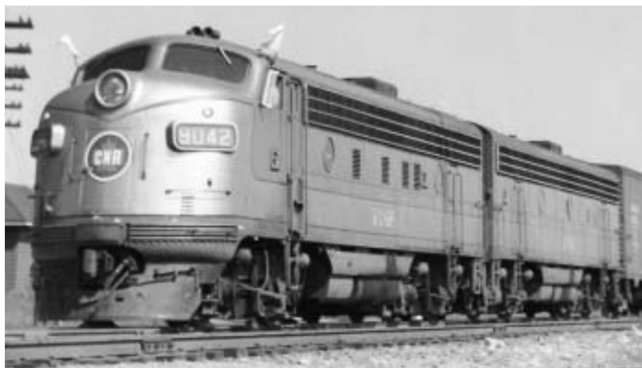
above: The round "CNR" monogram was applied to the noses of F-units and both ends of road switchers as per drawing 2H-26054. CNR F7A No. 9042 and a B-unit were at Turcot West in September 1952. No. 9042 was delivered from GMD in 1951 and was rebuilt as F7Au No. 9169 in October 1973. The unit is currently being restored by the Central B.C. Railway and Forest Museum in Prince George, B.C.—Al Paterson Collection
